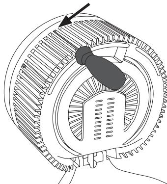
2. Turn the grille in the direction of the arrow to remove it.
