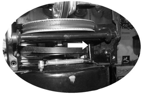
10. Pass thereafter the drive belt over the upper pulley. Untie the clutch lever on the right handle and refit the wire connected to the left handle (fig.4).
