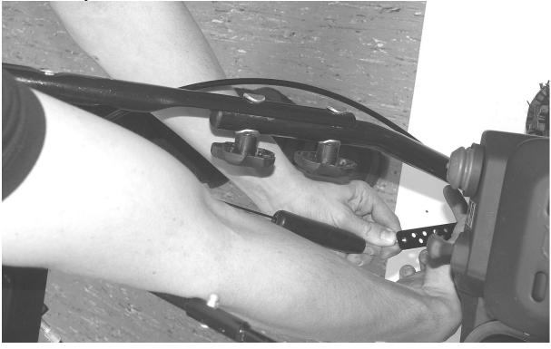
5. To access the drive belt the snow blower needs to be opened up in the middle. Return the snow blower to its normal upright position and remove the uppermost of the two bolts just behind the impeller housing on both sides. The two lower bolts do not need to be removed, just loosened (13 mm spanner).
