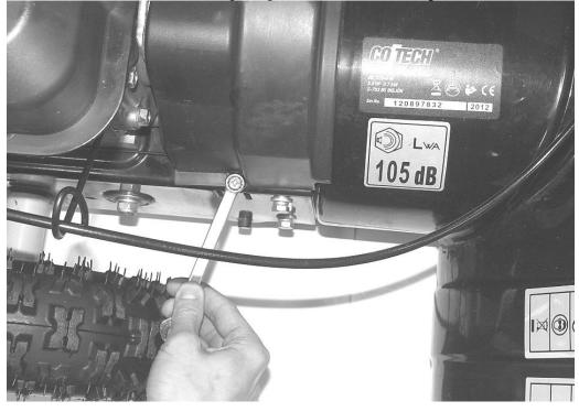
1. Remove the two bolts holding the plastic cover (10 mm spanner).
