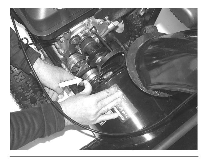
9. Pass the drive belt over the lower pulley once the guide wheel/brake has been moved. Note: This view is from below the snow blower.
