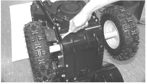
4. Slacken the auger drive clutch wire connected to the left handle. Remove the s-hook from the connector plate.
