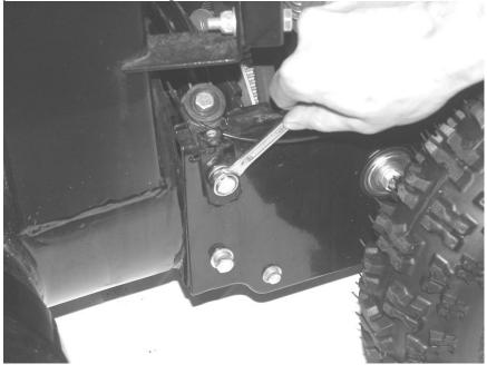
6. Tilt down the front and rear parts of the snow blower, pivoting on the two loosened bolts to create room for you to work on the now exposed drive belt pulleys.
