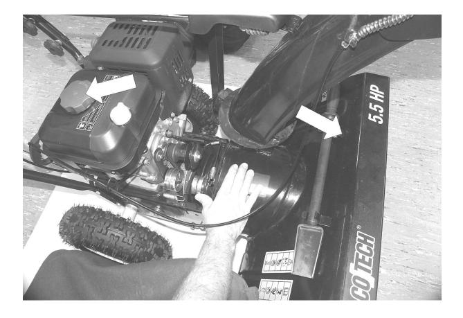
7. Squeeze the clutch lever on the right handle and tie it down with a cable tie or similar. This moves the drive wheel away from the belt pulley giving you more room to work.
