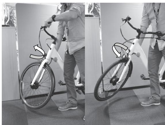
1. Hold the down tube (W2) with one hand, and lift the bicycle so that the front wheel (U) leaves the ground.
