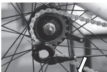
11. Lift the chain (X5) away from the rear sprocket (X7).
