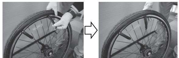
4. Use an additional one or two tyre levers at intervals of 10–15 cm, and continue until the entire side of the tyre comes away from the wheel rim.
