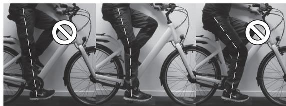
1. Rotate the crankset so that one pedal (X3) reaches its lowest point.
