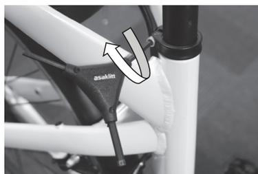
1. Loosen the socket head screw (5 mm) on the seat post clamp (L4).
