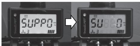
2. Press [**⏏**] repeatedly until "SUPPORT" appears momentarily on the display, followed by "SU" together with the value of the current setting from -15 to +15.
