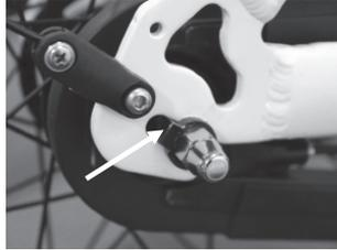
8. Centre the wheel between the chainstays, and lightly tighten the wheel nuts.
