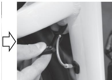
13. Try applying the brakes and check that the brakes work (see *Brakes* in the *Settings and adjustments* section).
