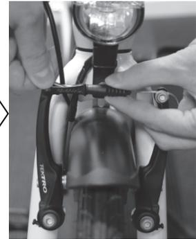
5. Try applying the brakes and check that the brakes work (see *Brakes* in the *Settings and adjustments* section).
