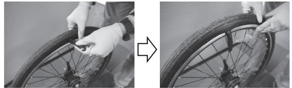
3. At the point opposite the valve, insert a tyre lever beneath the edge of the tyre. Pry up the edge of the tyre and fix the tyre lever to one of the spokes.
