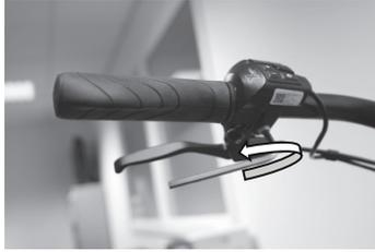
2. Move the levers inwards or outwards along the handlebars, and/or move the levers to the required angle.
