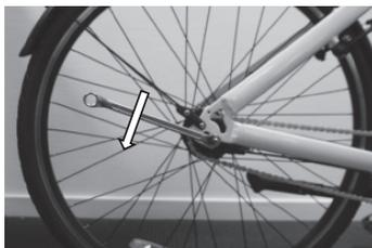
8. Push the wheel downwards/ forwards so that the wheel axle comes away from the rear fork (W8).
