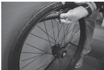
5. Hold the valve in place and push the side of the tyre around the valve over the wheel rim.
