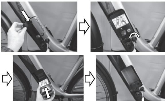
1. Push the catch downwards and remove the battery cover.
