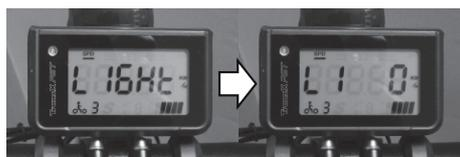
2. Press [**⏏**] until "LI6H..." appears momentarily on the display, followed by "LI" together with the value of the current setting from -15 to +15.
