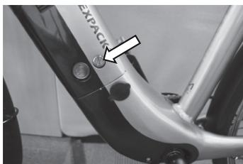
If you do not turn the electrical system off using the power switch on the frame/battery, you can turn it off (and on) using the control unit on the handlebars.
