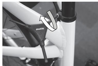
1. Lossa sadelstolpeklämmans (L4) insexskruv (5 mm).
