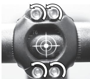
2. Twist the handlebars up/down to the desired angle and make sure that the stem is centred on the handlebars.
