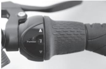
1. Turn the gear shifter to position 1.
