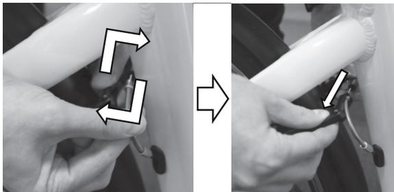
12. Press the brake arms in against the wheel rim, hook the cable guide onto the link, and press the gaiter into place.
