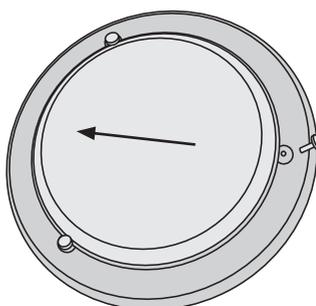
5. Remove one of the diffuser retaining screws, carefully slide the diffuser in under the other two screws and then refit the first screw.
