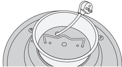
1. Connect the incoming feed cable or lamp lead with plug (sold separately) to the terminal block, attach the hanging bracket and fit the included spacer ring.
