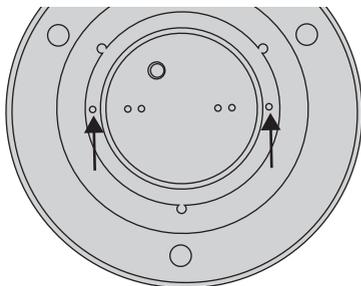
1. Use the mounting holes in the light fitting to mark out where the holes in the ceiling are to be drilled.
