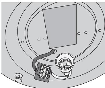
3. Connect the incoming feed cable to the terminal block. Use the three wire insulation sleeves (included) if you have three separate wires coming from the ceiling.
