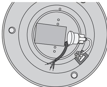
2. Feed the incoming feed cable through the hole in the light fitting and screw the light fitting directly to the ceiling using suitable fasteners.
