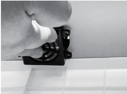
17. Attach the air filter under the fan.
