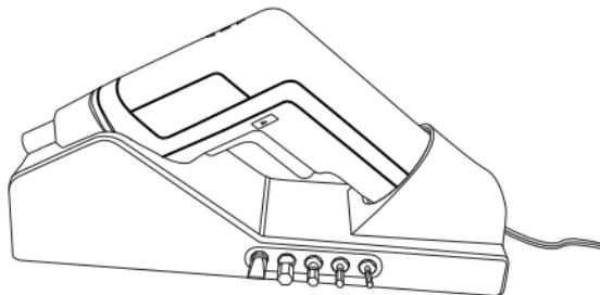
4. Remove the screwdriver from the cradle by lifting it in the direction of the arrow.
