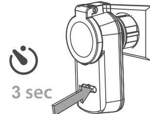
3. The LED in the button will start flashing slowly. The receiver is now ready to be paired with a remote control/transmitter. **Note:** The button will begin to flash after it has been released. If the button is flashing when it is being pressed, the pairing will not be successful.
