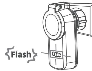
4. Remove the plastic tab to activate the battery in the remote control.
