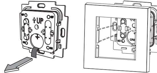
3. Remove the plastic tab to activate the battery.
