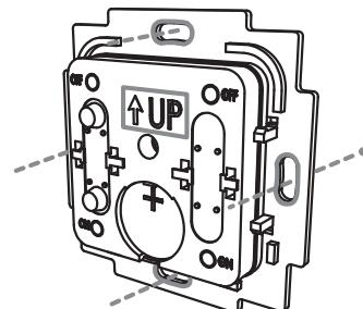
1. Remove the push button and frame from the switch module.
