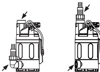
The universal hose union is fitted with a 38 mm (1½") and 25 mm (1") diameter barbed hose connectors and a 1" male threaded hose connector. 38 mm hoses provide the best capacity.
