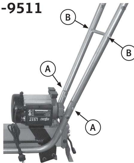
3. First fit the extensions to the legs on the motor side using the screws labelled **A**. Then screw the cross member between the legs using the screws labelled **B** (do not fully tighten the screws yet).
