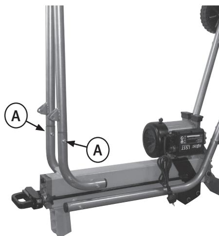
5. Fit the extensions to the legs on the other side of the log splitter using the screws labelled **A**.
