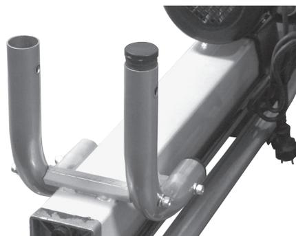
2. Turn the log splitter upside down, detach the wheels and remove the plugs from the ends of the legs.
