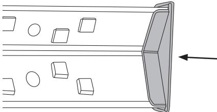
2. Start with the lowest shelf and push the hooks on the end shelf supports into the slots on the uprights.
