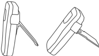
**Note:** If the stand is over-extended it will release its grip from its mount to prevent damage. Refit the stand back into its mount and it will function normally again.
