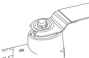
3. Turn the locking lever back so that it stands at 90° from the front of the machine. The locking washer cannot fall from the tool mount when the locking lever is in this position.
