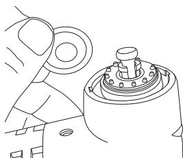
3. Remove the locking washer from the tool mount.
