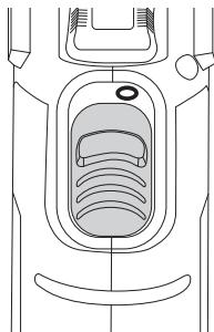
2. Start the multi-tool by sliding the power switch to the **1** position (on).
